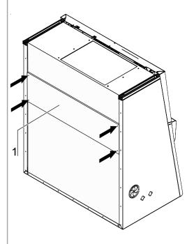
Fig. 11 Unlocking the transport protection
